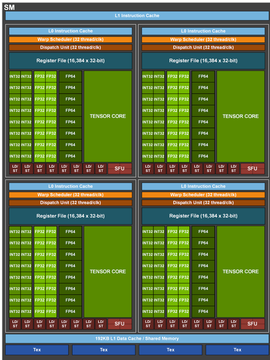
Figure 10.4. A single SM showing multiple cores contained within.
